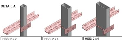
PLATE: 2" x 6" x 1/4" BOLT: Carriage bolt 1/4"ø - 3" long or Treaded rod 5/16"ø - 3" long PIPE: 1/2" STD (0.84"ø OD)
